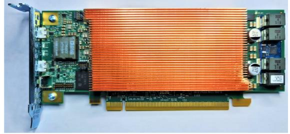
Penguin Computing production ET-SOC-1 PCle card with and without heatsink
