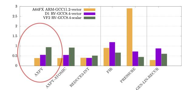
RISC-V timing normalised against D1 scalar A64FX vector timing normalised against A64FX scalar Lower is better
